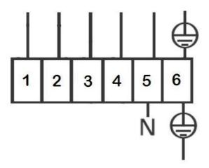
Incoming 240V active connects to terminals 1 thru 4 depending on speed required.
